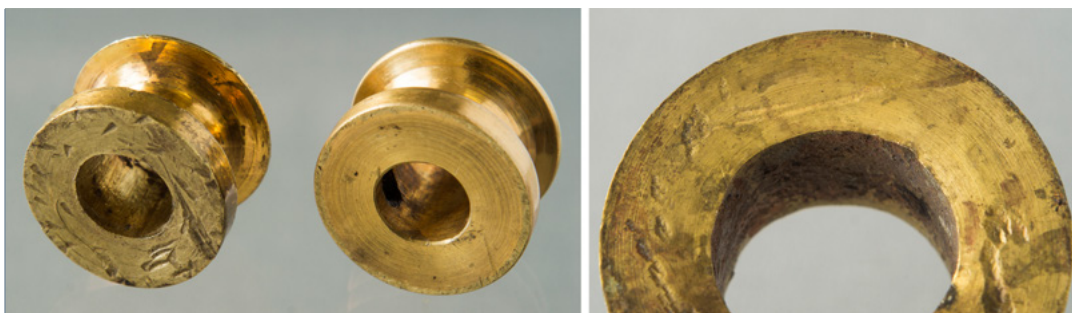
[fig. 30] Copper-alloy pieces with visible lathe lines.
