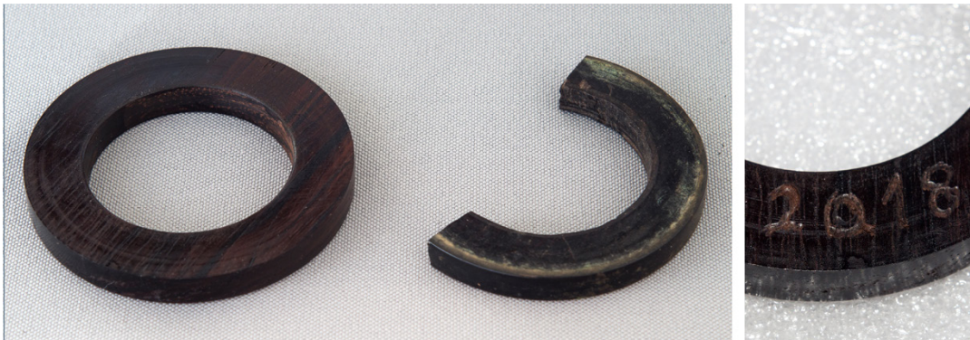
[fig. 54] The new piece and broken old one (D86) (left) engraved with the year it was made (right).
