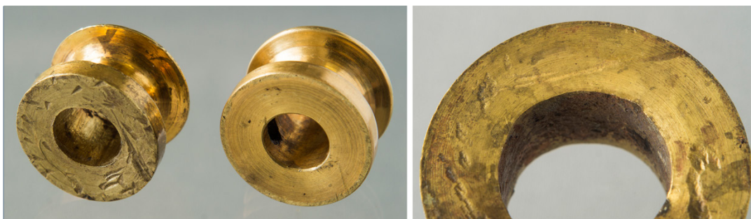
[fig. 30] Copper-alloy pieces with visible lathe lines.
