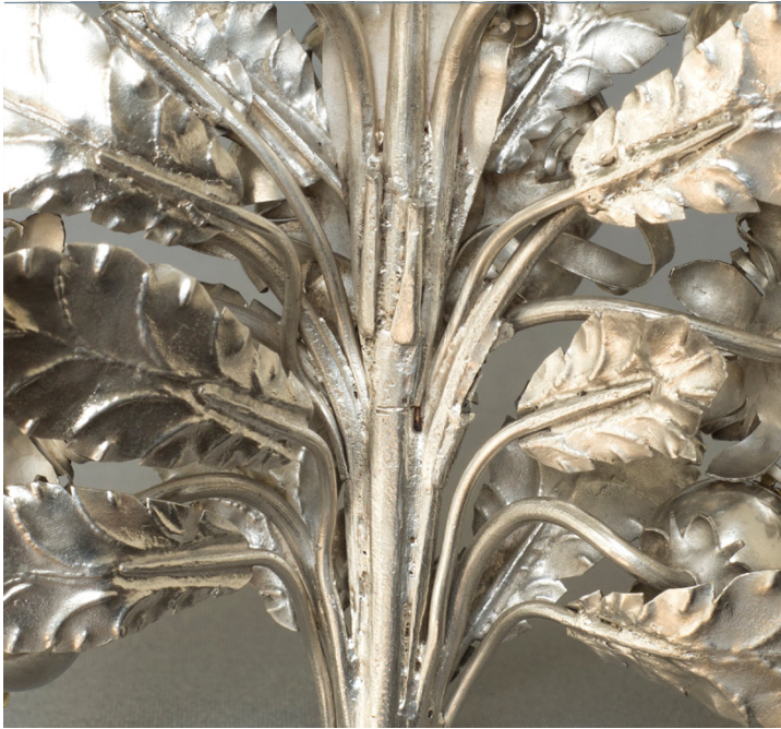
[fig. 23] Sloppy soldering of the stems and leaves on a bouquet of flowers and fruit (ER1).
